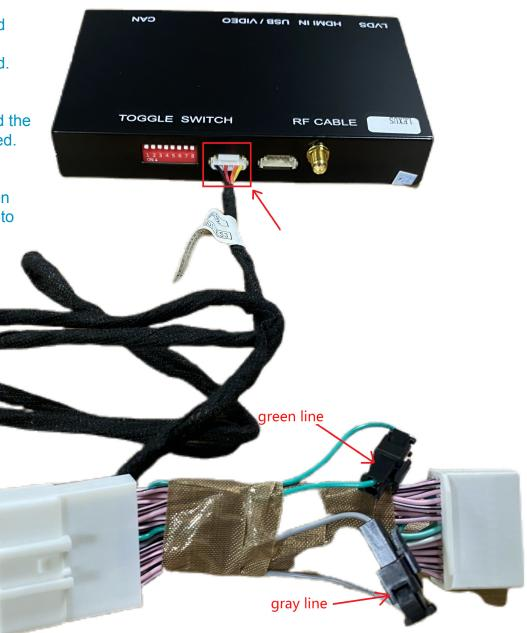
Plug the power cord removed from the original car screen Connect the screen jack
